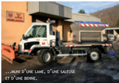
...MUNI D'UNE LAME, D'UNE SALEUSE ET D'UNE BENNE.
